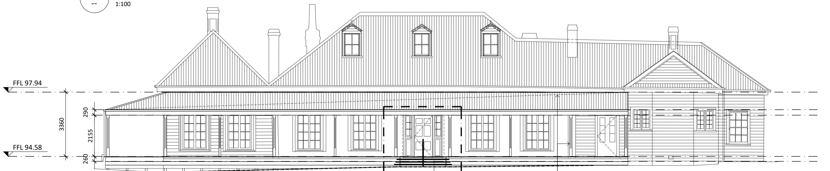
04 SOUTH ELEVATION - PROPOSED VERANDAH 1:100
