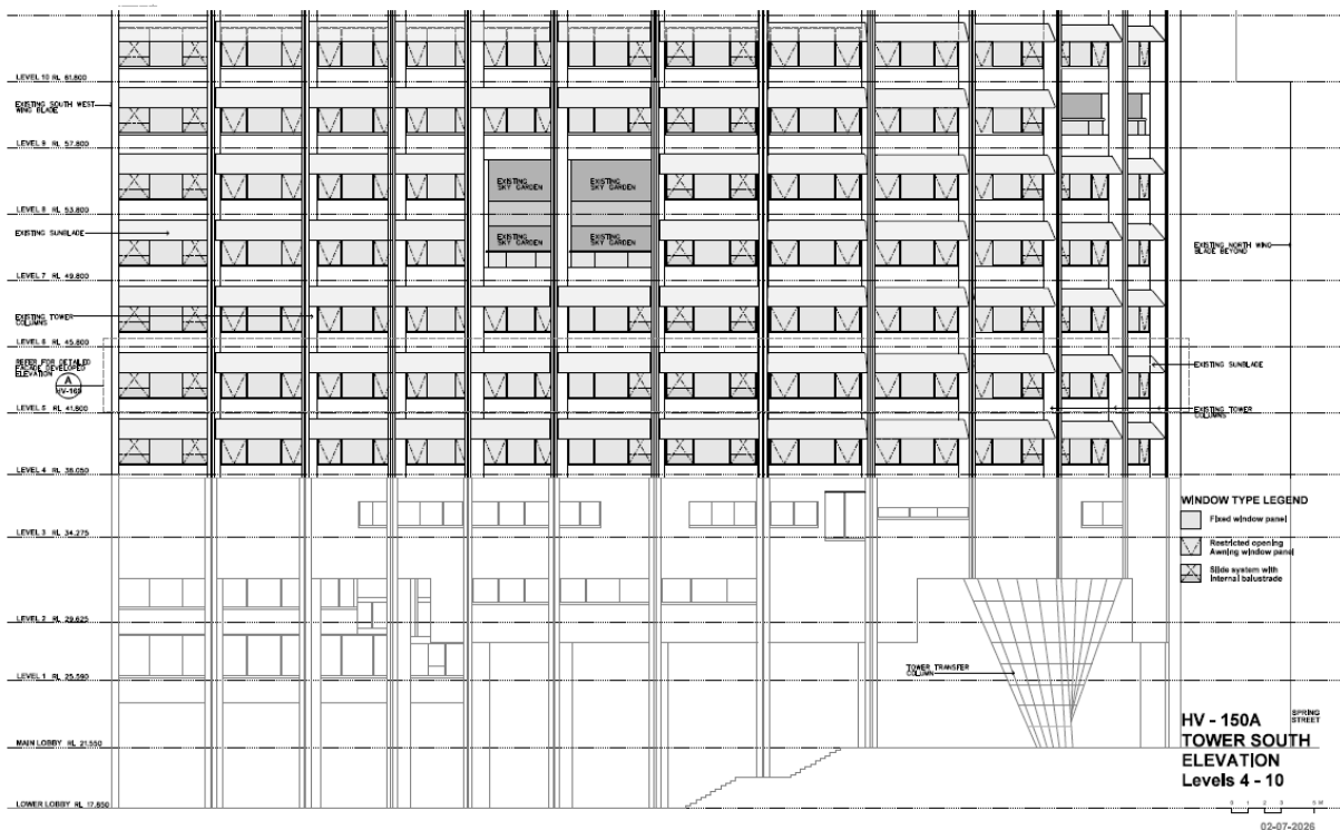
Figure 43 South elevation showing replacement glazing applied to the lower levels Source: HSA – HV-150A Tower South Elevation, Levels 4-10
