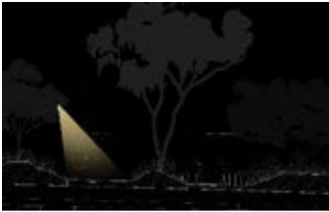
Post-top dark-sky lighting along primary pathways provide warm and well distributed illumination, whilst minimising impact on flora and fauna.
