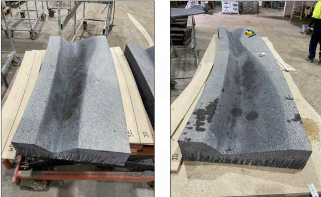
Figure 3.2 Sample of bluestone rill similar to that proposed – preliminary design work. (Source: GbLA, 2023)
