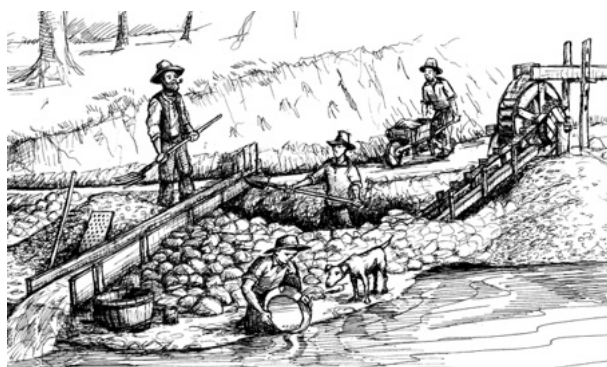
Figure A3.1: River claim, using a Californian pump to drain workings.
