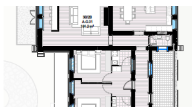
Figure 85 Example of wall stepped to avoid window
