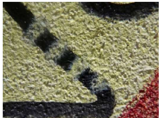
Tests done by conservators to identify the best solvents to remove the graffiti without damaging the mural paint
