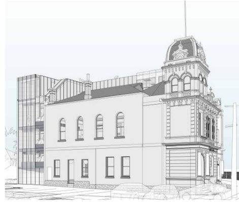
Figure 7: Extract of drawing A3-803 from updated HV02 set. Proposed view from Little Chapel Street, looking south. The service equipment is largely concealed by the original building's roof ridge line and only has negligible visibility from oblique views. Source: Trethowan Architecture, 2025.
