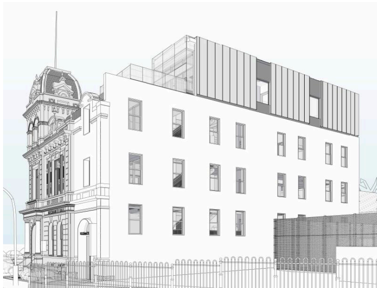
Figure 9: Extract of drawing A3-803 from the updated HV02 set, showing the southern elevation of the building. The proposed additional level is modest in comparison to the existing fabric. Source: Trethowan Architecture, 2025.
