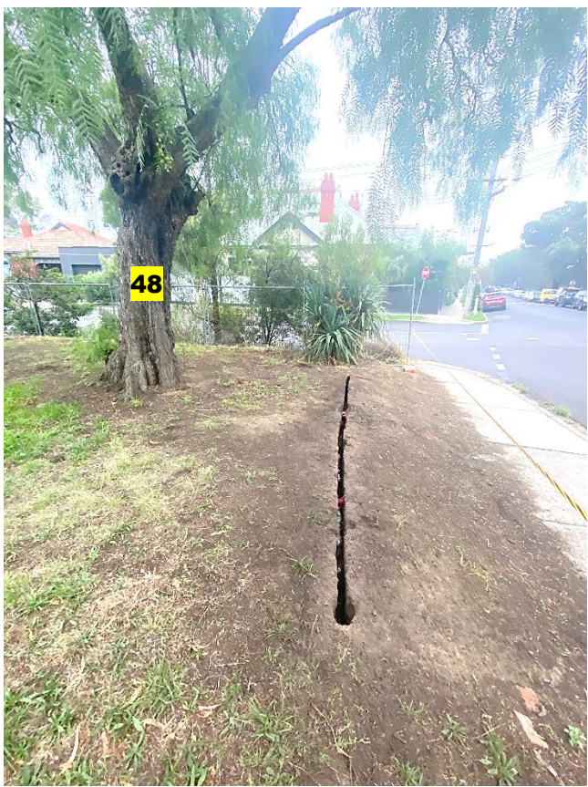
Image 12: Tree 48 two rots located 20mm, 35mm.
