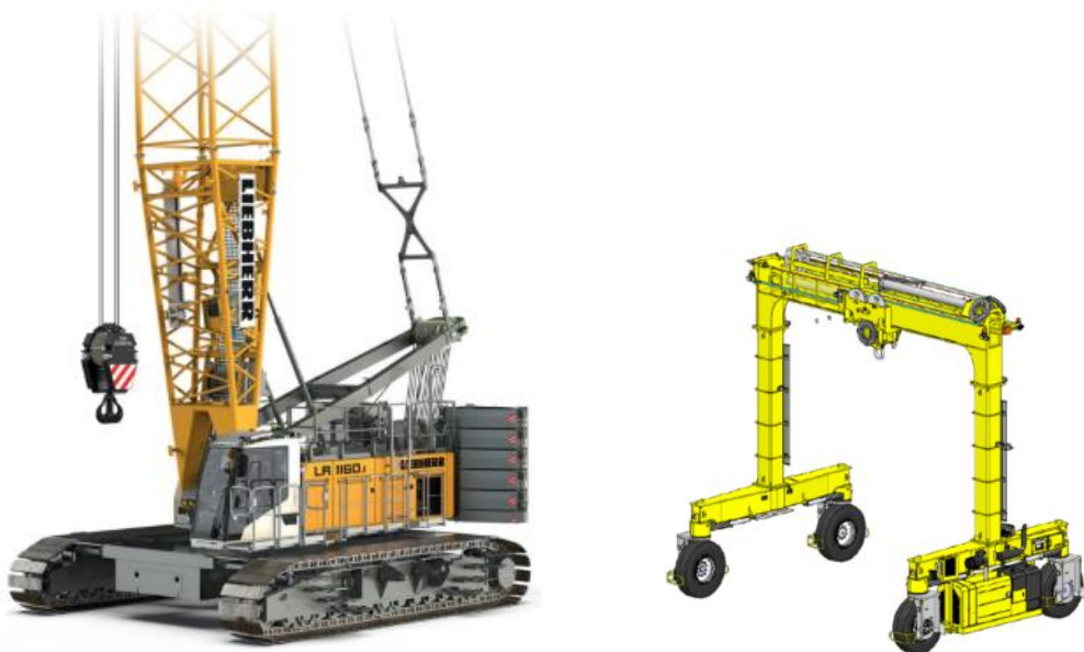
Figure 3-6. Example of 160 tonne crawler crane and mobile gantry (Confidential contractor 2025)
