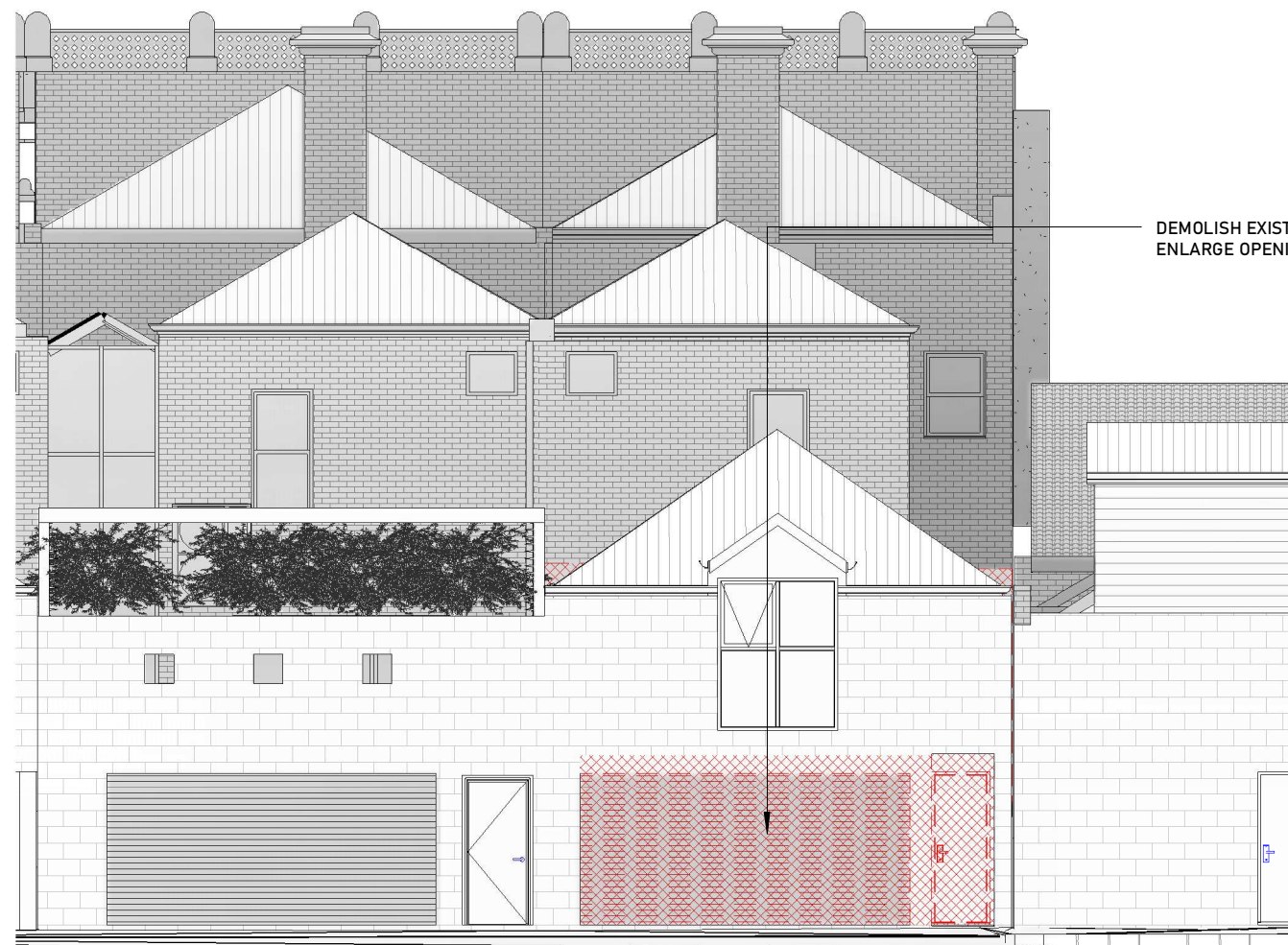
5 South Elevation Bevan Street Demolition 1: 100
