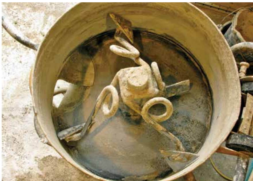
Figure 45: Forced action mixer. Looking down into the mixing pan of a forced action (screed) mixer in which the blades rotate about a vertical axis. The relatively small blades force the lime and sand particles together in a way not achieved with conventional rotary mixers.
