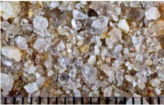
Figure 19: Grading of sands. The sand on the left is well graded. It has a wide range of particle sizes from very coarse through coarse, medium, fine and very fine. The sand on the right is poorly graded, with a relatively uniform (fine to medium) particle size. Each division on the scales in these photographs is 1 mm; each image is about 20 mm across.
