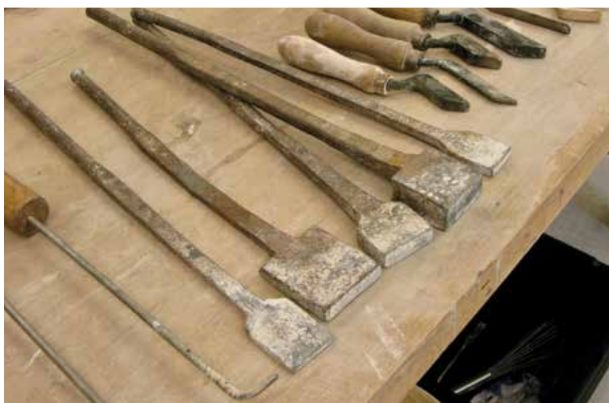
Figure 74: Steel tamping or deep-packing tools. While the aim is tightly compacted mortar, tamping with these heavy, purpose-made tools needs to be done with care, as too much force will break the bond of the remaining joint. Other packing devices include pieces of wood or plywood for narrow joints. Mortars must be relatively dry and stiff if they are to take up the load of overlying masonry and weatherproof the wall. The outer part of the joint is finished in the way described in the previous chapters.
