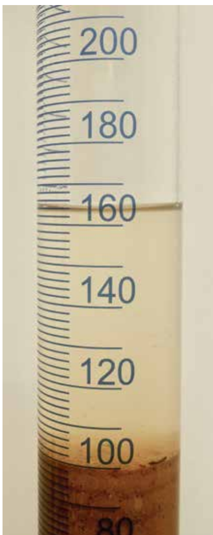
Figure 25: Establishing the void ratio of a sand. Using a measuring cylinder, 100 ml of dry sand is poured onto 100 ml of water, the difference from 200 ml is the amount of water now filling the voids. This is expressed as a percentage, in this case 36%.
