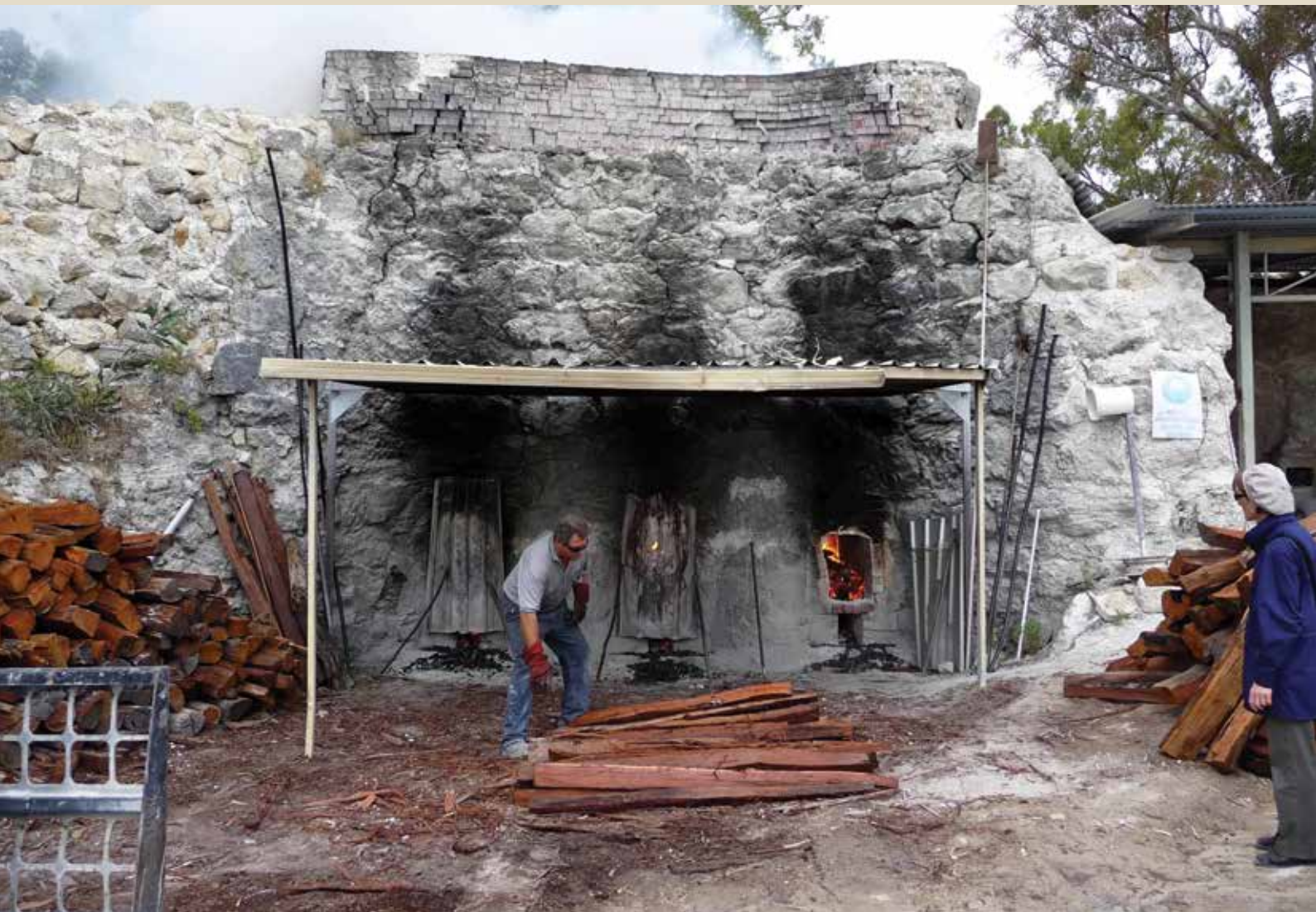
Figure 7: Traditional lime burning. A lime kiln at Susac Lime Supply, Carabooda, north of Perth, Western Australia. This may be the last such lime kiln operating in Australia: most had ceased production by World War II.
