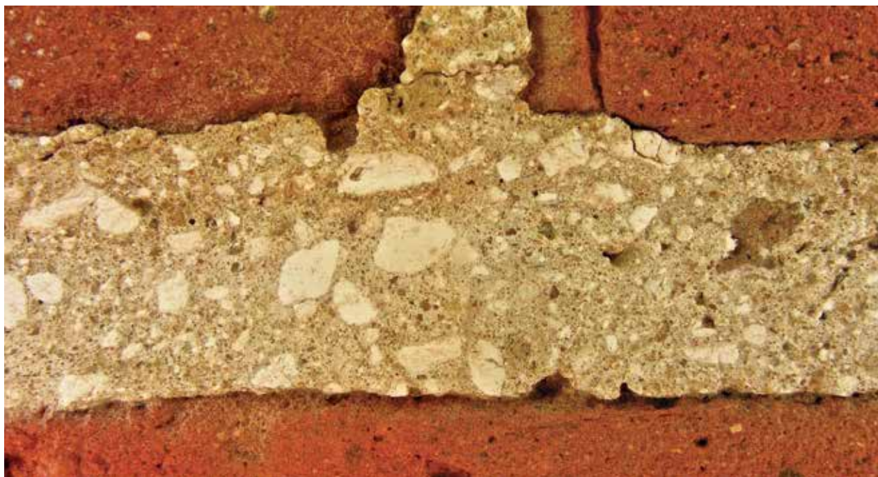
Figure 42: An 1840s mortar.
