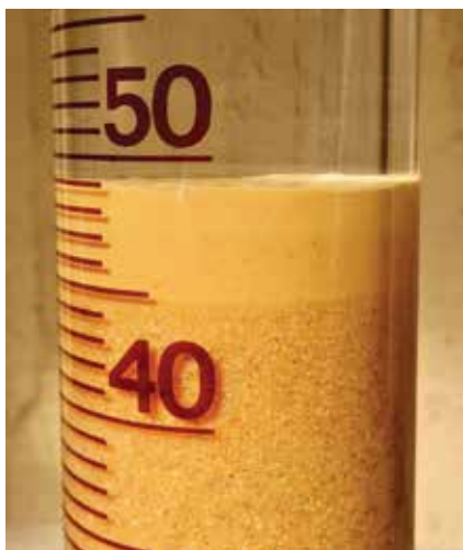
Figure 24: Settling test. A clay layer settled on top of a fine sand after shaking in water. At 9% clay this sand is not suitable for use in mortars.
