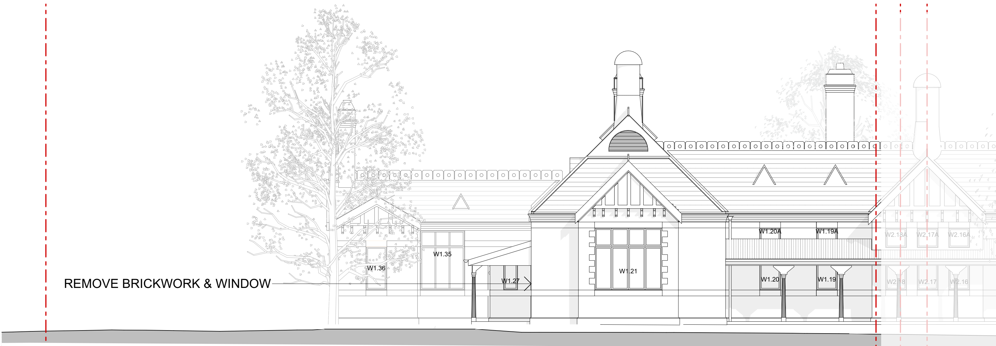
EAST ELEVATION - DEMOLITION 1:100 @A1 /1:200 @A3
