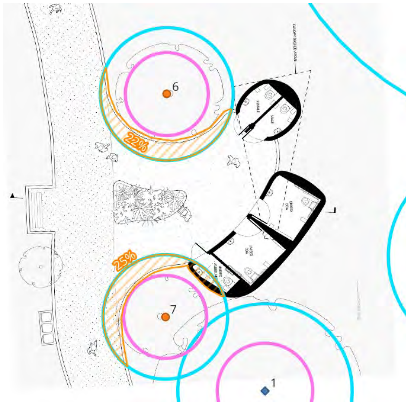
Figure 10. An image of the NRZ calculation for Trees 6 and 7 with the orange showing the proposed impacts to NRZs. Civica ArborSafe, February 2026.
