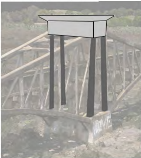
1. At rest condition. Rigid pier legs (4x) provide support to truss and pier head
