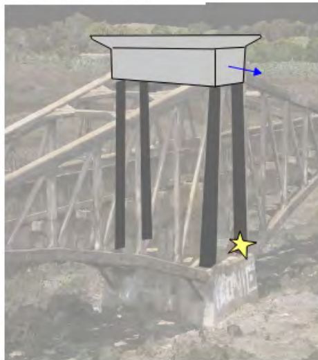
2. Single pier leg failure occurs. Minor sideways movement
