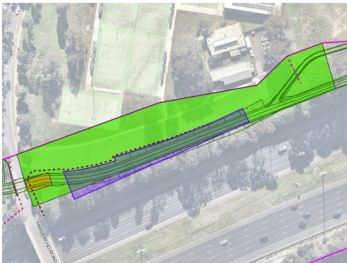
Figure 103: Location of the Fairlea Reserve Netball Courts carpark earth mound in relation to the identified areas of low (green) and moderate (orange) archaeological potential
