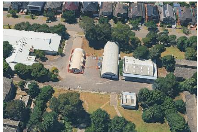
Figure 31. Nissen Hut (centre left) and Romney Hut (centre right), Former Maribyrnong Migrant Hostel [part]. (Source: Google Maps, aerial image dated 2005)
