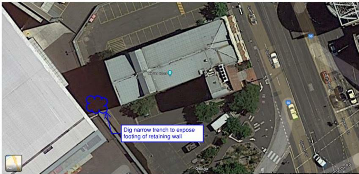
Figure 2: Location of narrow test pit along site boundary to investigate the footing of the retaining wall on the neighbouring site
