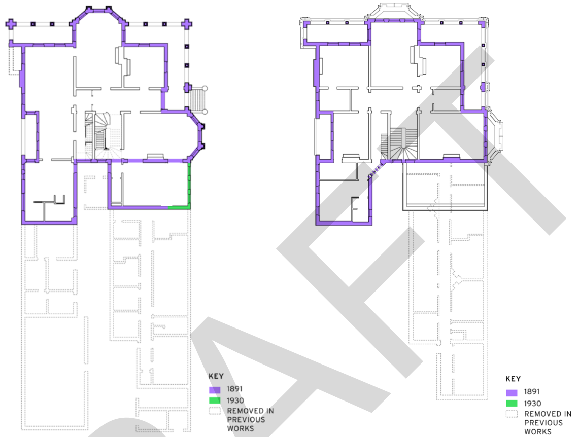
Figure 6 Plan showing the surviving extent of the of the ground floor (left) and first floor (right) of the mansion, as shown by the development era indicated (north is at left) Source: Lovell Chen
