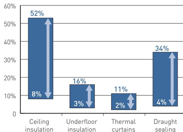
Figure 4: Reductions in heating and cooling energy when selected interventions are applied.
