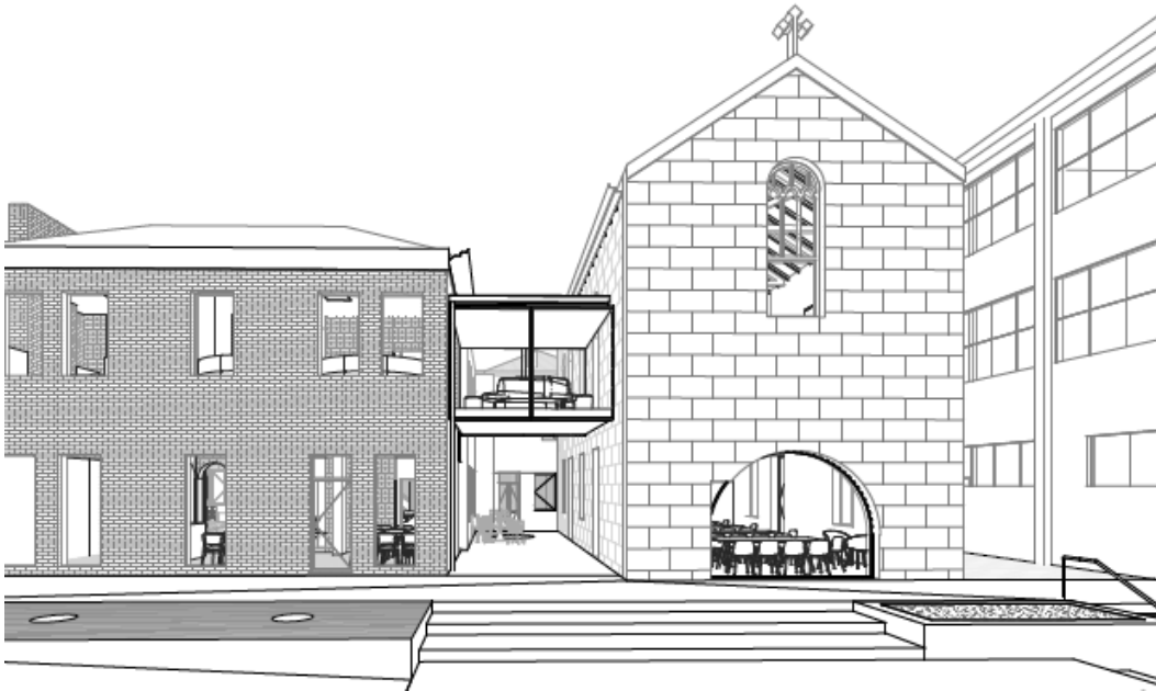
Figure 9 Perspective of the new glazed link on the first floor between Twelve Sisters House and Goold residence Source: PMDL-McGlashan Everist
