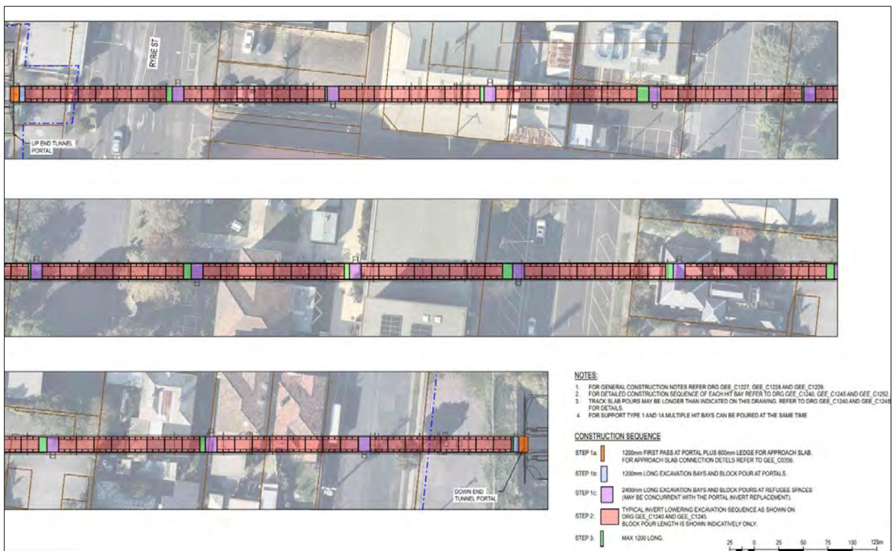
FIGURE 17: PLAN SHOWING CONSTRUCTION SEQUENCE. (SOURCE: AURECON/VLINE)
