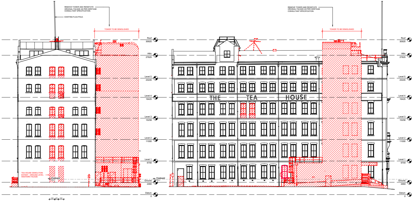
Proposed Demolition West Elevation
