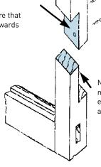
New timber chosen to match line and density of existing grain as closely as possible.
