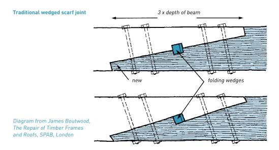
The timber species and moisture content of the new timber need to be carefully matched with the old to avoid differential movement. For clear-finished joinery, the colour and grain direction of the repair also need to be matched, and the new piece fitted to the old with a hairline joint.
