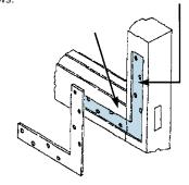
Bracket let into (or fixed on surface of) timber on inner face of sash or casement.
