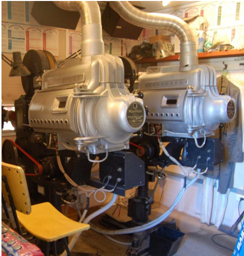
Early projectors still in use in the Swanpool Cinema with arc light ventilation tubes.
